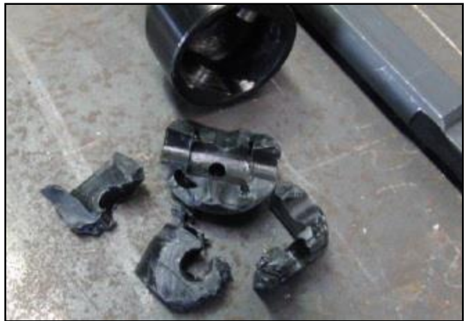
Collapsed remains of the plastic tilt mechanism in a “Helix” column which caused complete steering failure.
